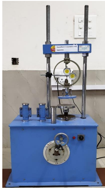
Figure 1: Experimental setup for unconfined compression test
