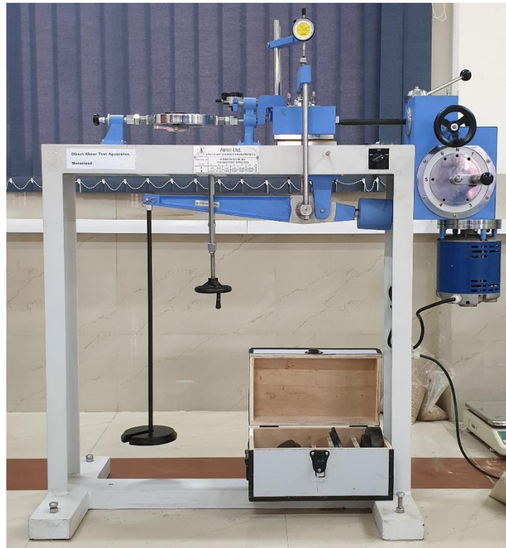
Figure1: Direct shear test setup
